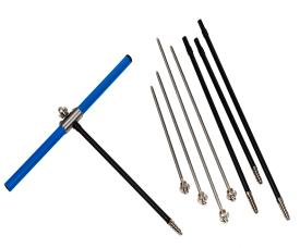
Never store your increment borer wet and dirty. Never drill with the extractor inserted in the borer
